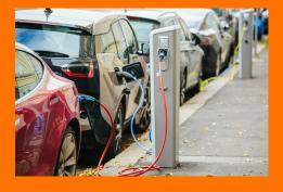
Council, to investigate solutions to this issue. The grant provided funding to develop a prototype technology designed to tap into existing streetlight infrastructure for curbside EV charging, lowering installation costs for curbside EV chargers compared to chargers that require the installation of new electrical infrastructure. EPIC collaborated with Duke Energy to develop a prototype for a pole-mounted EV charger, called PoleVolt, and deployed two pilot chargers in the City of Charlotte.
