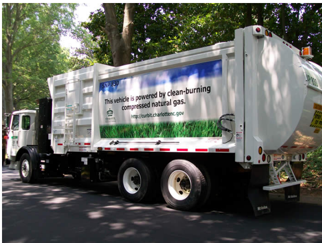
City of Charlotte’s Solid Waste Services has ten compressed natural gas (CNG) automated refuse vehicles in service.
